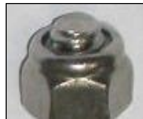
Figure 2. Incorrect - too tight. Screw extends beyond edge of nut.
