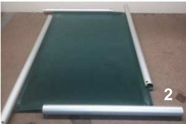
Insert fabric sleeves into the channel on each length of pipe.
